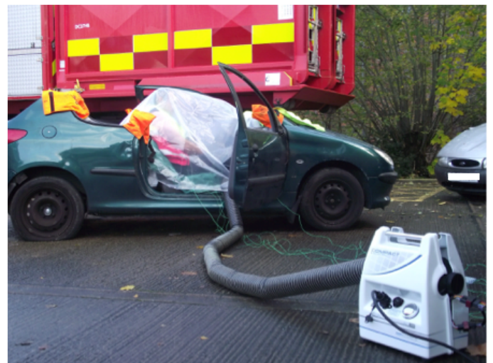
Figure 1. (Forced Air Warming in Action): Volunteer underneath a plastic cover, which is used by HWFRS to protect entrapped victims from debris during extrication; heated air is blown underneath the cover using a Polarn 4000 (Eberspächer, Germany) outdoor heater.
