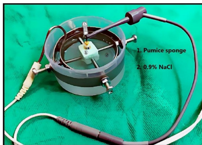
Figure 1. Fixation device showing the root placed in a pumice sponge and fixed with four long screws
