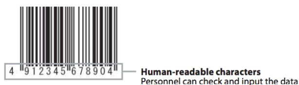
Figure 2. Bar code, read by laser scanners
