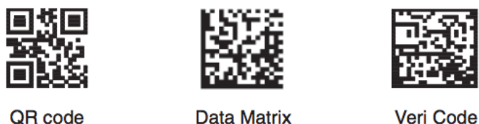
Figure 3. QR code has a square frame, for reliable position detection and more efficient data storage than the simpler bar-code; its speed is its most important quality. These machine codes are totally “demotive”, incapable of encoding emotive states
