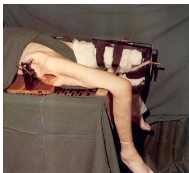
Image 1. Device used to test stability of the Hip Joint showing the pelvis fixed and protractors to measure the angle of flexion/extension, adduction/abduction and internal rotation/external rotations (Courtesy: Photograph reproduced with the kind permission of Injury/Elsevier).
