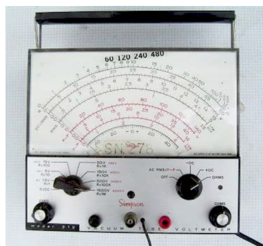
Figure 1. A typical vacuum tube voltmeter. The scale for resistance increases to the right and diminishes towards the left, which is opposite way to analogue multimeters. On this unit, the far right is a maximum value of 1,000 million Ohms.
