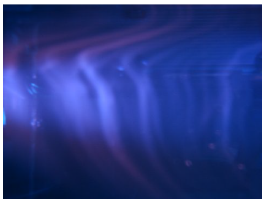
Figure 4. Standing wave patterns of scattered light in water with silver nanoparticles illuminated with a single 405 nm LED.
