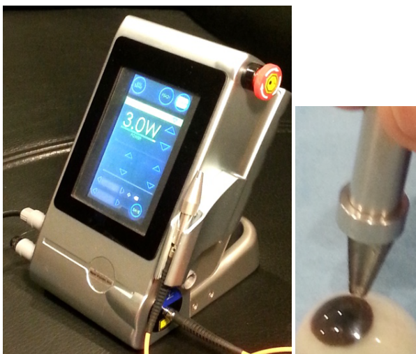
Figure 11. shows a diode laser (at 808 or 980 nm) for photocoagulation of the corneal tissue for glaucoma treatment, where a probe tip connected to the fiber is used to deliver the laser energy [31].
