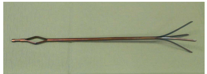
Figure 1a. FGL-nails with NiTi alloy, length 260 mm, diameter 2 mm
